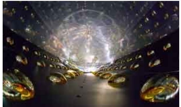
Photomultiplier tubes line a detector chamber at the Daya Bay Reactor Neutrino Experiment in Guangdong province, China.
